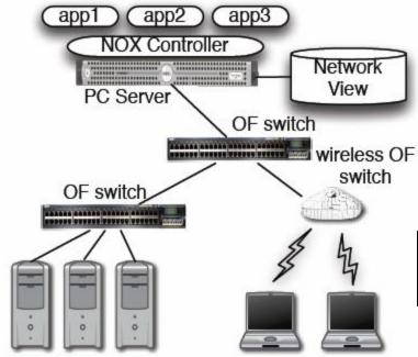
OpenFlow is used to control switches
