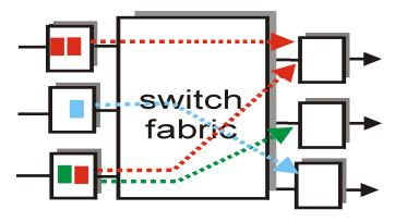
output port contention at time t - only one red packet can be transferred
