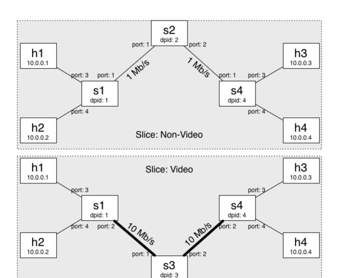
c. (15P) FlowVisor has to process the so-called *new flow messages*, i.e., those messages that have to be forwarded to the controller in case of a table-miss at a OpenFlow switch. Here, FlowVisor has to determine the correct recipient controller of these messages before forwarding the new flow message to that controller.
