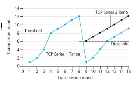
Tahoe always down to 1MSS, Reno distinguishes: 3 duplicate ACKs-> go down to 50% then CA, timeout -> go down to 1MSS
