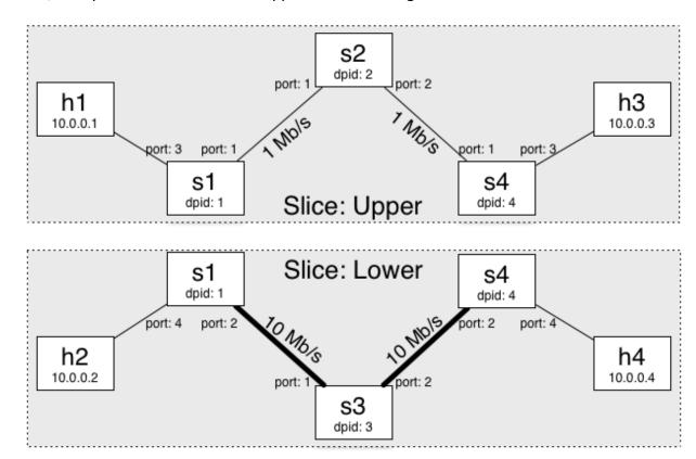
In short, this slice arrangement allows traffic to be sent from h1 to h3 and h2 to h4 (and viceversa) only, even though the topology itself would allow sending traffic between arbitrary pairs of hosts.
