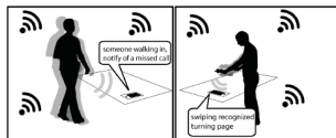
Fig. 1: Activity obtained from RSSI-signatures. Two example use-cases: user walking in with the smartphone implicitly reacting (left) and a no-touch explicit interaction (right).
