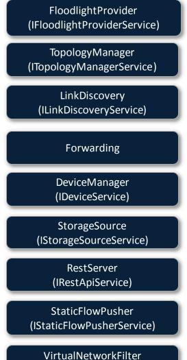
VirtualNetworkFilter (IVirtualNetworkFilterService)  Floodlight is a collection of modules
