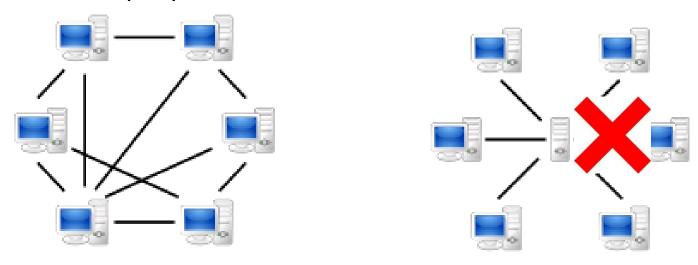
The sharing of computer resources by direct exchange, rather than requiring the intermediation of a centralized server.
