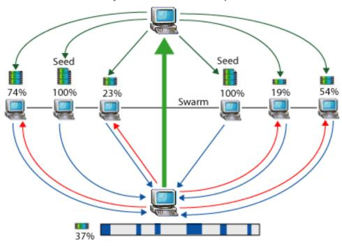
Computer with BitTorrent client software receives and sends multiple pieces of the file simultaneously.
